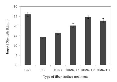
FIGURE 5. Impact strength of TPNR and (NR/HDPE)/RH (90:10 v/v) composite, plotted as a function of RH surface treatment
