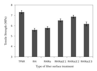
FIGURE 3. Tensile strength of TPNR and (NR/HDPE)/RH (90:10 v/v) composite, plotted as a function of RH surface treatment
