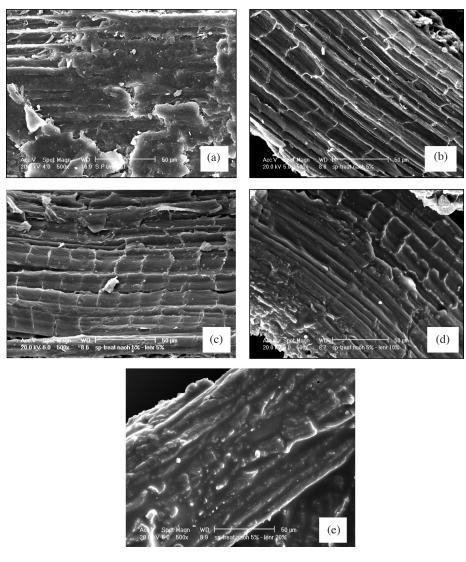
FIGURE 2. SEM micrographs of RH (a) RHi, (b) RHiNa, (c) RHiNaLE 1, (d) RHiNaLE 2 and (e) RHiNaLE 3
