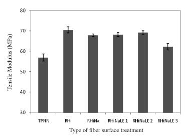
FIGURE 4. Tensile modulus of TPNR and (NR/HDPE)/RH (90:10 v/v) composite, plotted as a function of RH surface treatment
